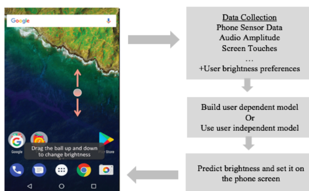
Figure 4.3: GUI part of the phone (on the left): sliding bar on the screen to collect brightness preferences and background service functions from data collection to brightness settings (on the right).
